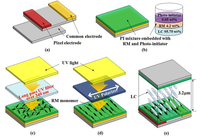
**Figure 2.** Schematic diagram of the fabrication process for achieving the strong anchoring energy of a photo-alignment layer.
