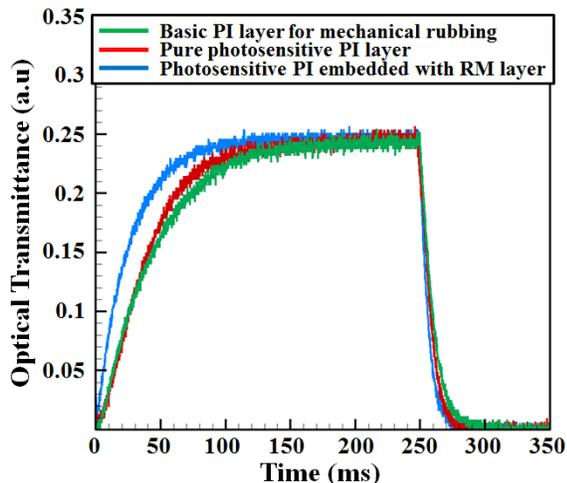
**Figure 4.** The calculated optical response time of an IPS LC cell for three alignment samples: a polymer films for mechanical rubbing, a pure photosensitive polymer materials and a proposed photosensitive polymer embedded with RMs.
