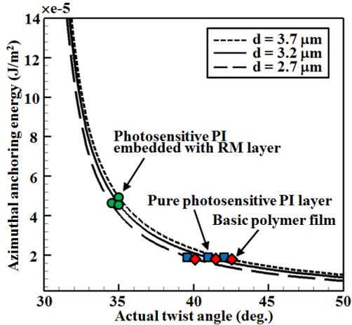
**Figure 3.** Comparison of the measured surface anchoring energy for three alignment sample: a polymer films for mechanical rubbing, a pure photosensitive polymer materials and a proposed photosensitive polymer embedded with RMs.
