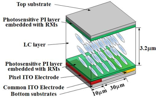
**Figure 1.** Schematic diagram of the modeled optical configuration of an IPS LC cell for experiments
