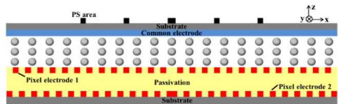
**Fig. 1.** (Color online) Structure of multi-electrode driving Fresnel LC Lens in which patterned pixel electrode 1 and 2 exists on bottom substrate and non-patterned common electrode exists on top substrate. The black areas on top substrate indicate locations for polymer stabilization.
