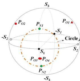
Fig. 3. (Color online) Polarization positions of light passing through the conventional wide-view PVA LC cell in normal and oblique directions in each domain at  $V = 2.5$  V.
