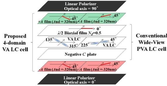
Fig. 6. (Color online) Proposed optical structure of the 4-D VA LC cell.
