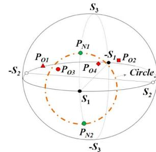
Fig. 5. (Color online) Polarization positions of light passing through the proposed 4-D VA LC cell in normal and oblique directions in each domain at  $V = 2.5$  V.
