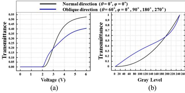
Fig. 2. (Color online) Calculated (a) V-T curve and (b)  $\gamma$  curve in a conventional wide-view PVA LC cell.
