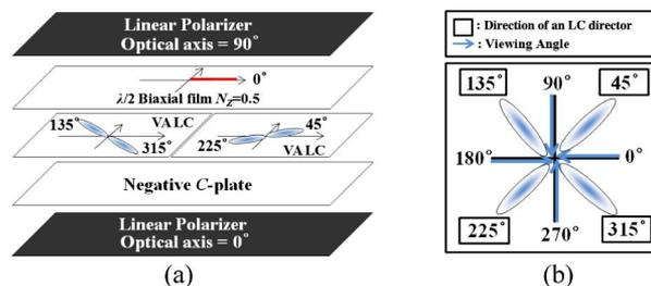
Fig. 1. (Color online) Example of the optical configuration of a conventional 4-D wide-view VA LC cell and the LC director configuration in each domain: (a) optical configuration and (b) LC director configuration.
