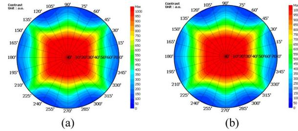
Fig. 8. (Color online) Comparison between the iso-contrast of (a) conventional wide-view PVA LC cell and (b) proposed 4-D VA LC cell.
