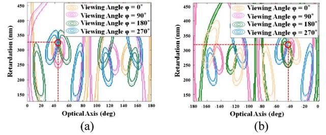
Fig. 4. (Color online) Calculated  $\Delta p$  of the pair of A plates at an all-viewing angle in (a)  $45^\circ$ ,  $225^\circ$  and (b)  $135^\circ$ ,  $315^\circ$  domain areas.
