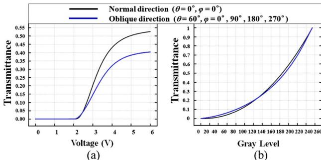
Fig. 7. (Color online) Calculated (a) V-T curve and (b)  $\gamma$  curve in the proposed wide-view 4-D VA LC cell.
