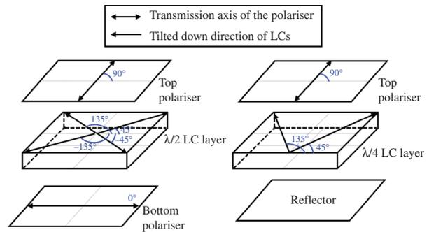
Figure 2. Optical cell configurations of the proposed transfective LCD: (a) T-part and (b) R-part.
