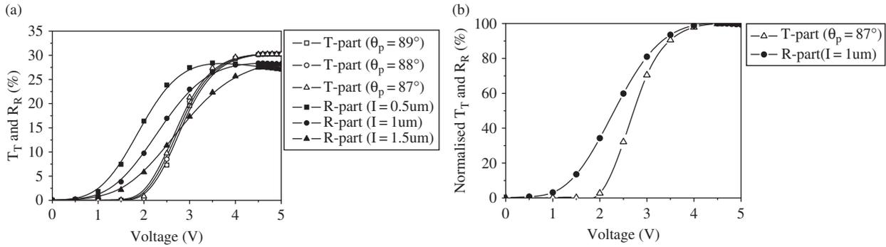
Figure 6. (a) Voltage-dependent  $R_R$  and  $T_T$  curves according to the pretilt angle and thickness of insulator layer in the T- and R-parts, respectively (b) normalized voltage-dependent  $R_R$  and  $T_T$  curves in the optimum gamma curve.
