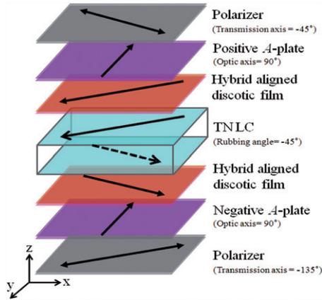
Figure 3. The optical configuration of the proposed WV-TN cell with a pair consisting of a negative *A*-plate and a positive *A*-plate. (The color version of this figure is included in the online version of the journal.)
