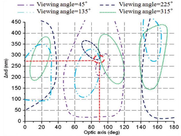
Figure 4. A parameter space of the polarization difference consisting of the optical axis and the retardation of the pair of *A*-plate parameters for optimization. (The color version of this figure is included in the online version of the journal.)
