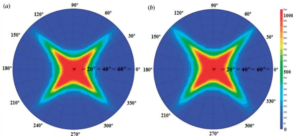
Figure 7. Comparison of the iso-contrast of (a) the conventional WV-TN cell (b) the proposed WV-TN cell. (The color version of this figure is included in the online version of the journal.)
