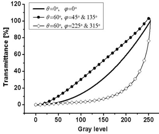
Figure 1. The calculated  $\gamma$ -curve of the conventional WV-TN cell. The solid line shows the  $\gamma$ -curve with index of 2.2.
