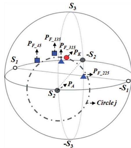
Figure 5. The polarization stats of light in front of the output polarizer on the Poincaré sphere with 1.8 V applied, which represents the 70th gray-level, in the proposed WV-TN cell. (The color version of this figure is included in the online version of the journal.)
