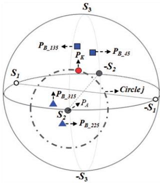
Figure 2. The polarization states of light in front of the output polarizer on the Poincaré sphere with 1.8 V applied, representing the 70th gray-level, in the conventional WV-TN cell. (The color version of this figure is included in the online version of the journal.)
