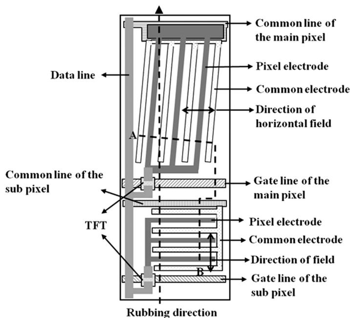
**Figure 1.** Schematic pixel structure of proposed viewing angle controllable LCD using IPS mode.
