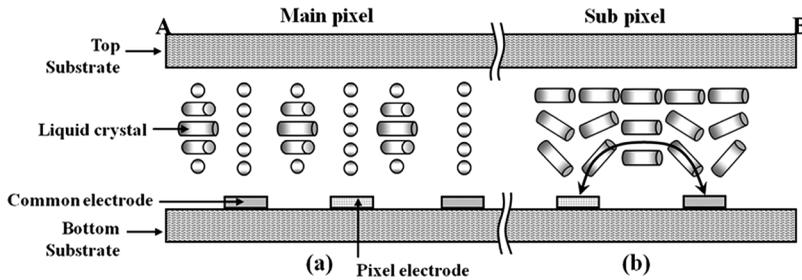
**Figure 2.** Cross sectional view of the viewing angle controllable LCD with LC profile in presence of an applied voltage in (a) main and (b) sub pixels.
