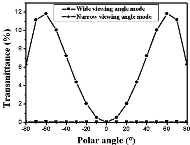
**Figure 4.** Calculated light leakage along horizontal direction as a function of polar angle in, wide at an applied voltage of 10 V and narrow viewing angle modes in absence of applied voltage.
