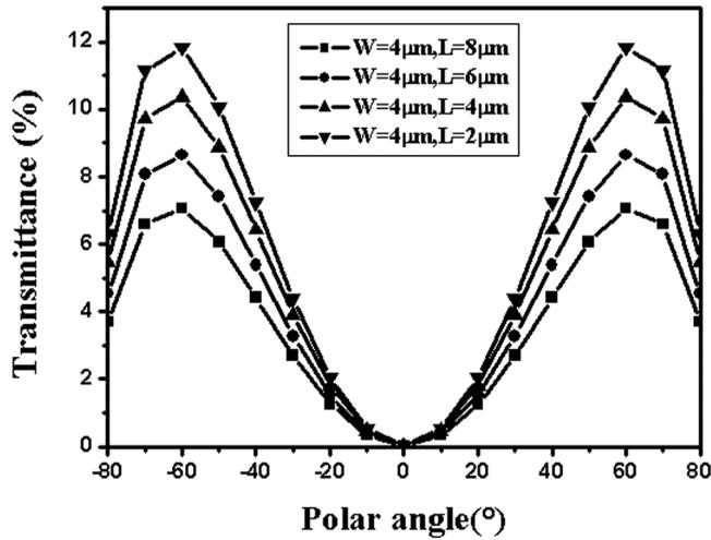
**Figure 3.** Calculated light leakage along horizontal direction as a function of polar angle with different electrode conditions under the action of an applied fixed voltage of 10 V.
