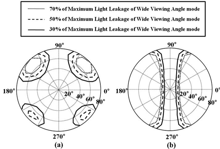
**Figure 5.** Calculated iso-luminance curves of dark state in (a) wide and (b) narrow viewing angle modes.
