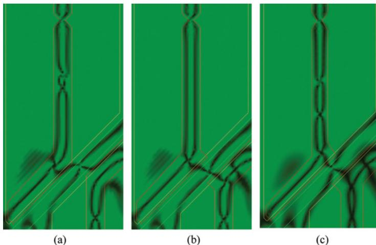
**Figure 6.** Calculated optical transmittance as a function of the width of the slit: (a) the conventional cell with  $8\ \mu\text{m}$  of the slit width, (b) the proposed cell with  $8\ \mu\text{m}$  of the slit width, (c) the proposed cell with  $7\ \mu\text{m}$  of the slit width. (Figure appears in color online.)
