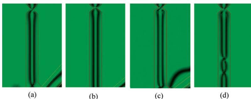
**Figure 5.** Calculated optical transmittance as a function of the length of the slit: (a) reference ( $20\ \mu\text{m}$ ), (b)  $25\ \mu\text{m}$ , (c)  $30\ \mu\text{m}$ , (d)  $35\ \mu\text{m}$ . (Figure appears in color online.)
