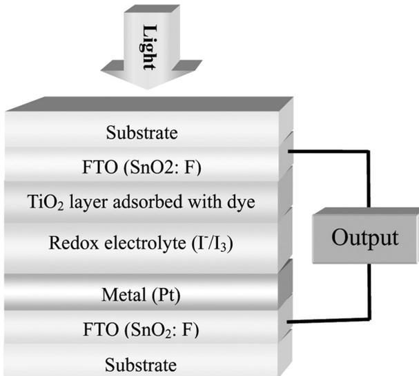
**FIGURE 1** Structure of a dye-sensitized solar sell.
