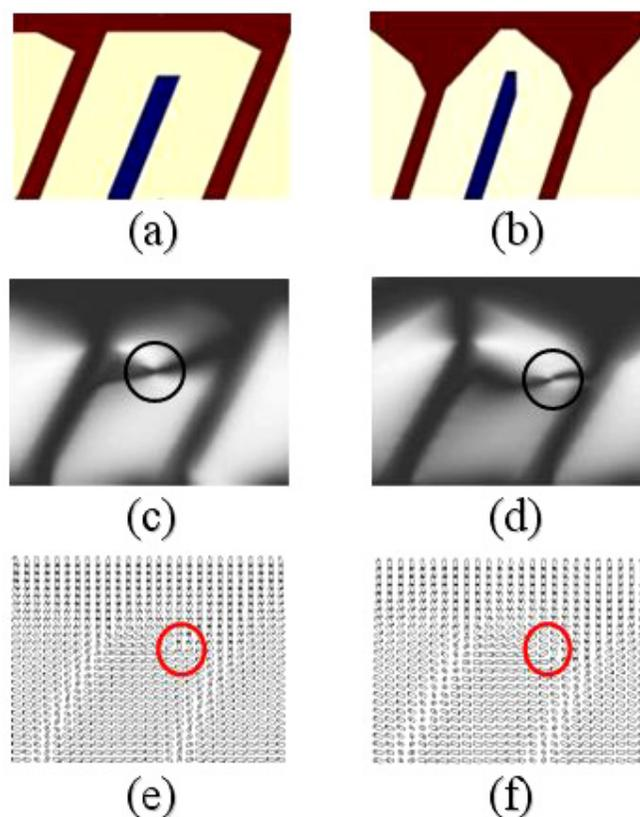
**FIGURE 5** — The shape of the electrode edge and the calculated optical transmittance: (a) the conventional structure, (b) the proposed structure, (c) the optical transmittance of the conventional structure, (d) the optical transmittance of proposed structure, (e) the calculated director profile around the edge of the conventional electrode, and (f) the calculated director profile around the edge of the proposed electrode.
