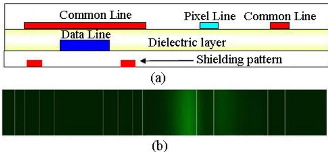
**FIGURE 2** — Improved light leakage by using the proposed electrode structure for bulk active areas: (a) the electrode structure, (b) calculated optical transmittance in the dark state.
