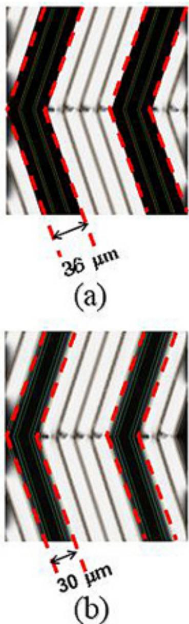
**FIGURE 4** — Comparison of the calculated optical intensity between the conventional LC cell and the proposed LC cell: (a) the calculated optical intensity of the conventional LC cell, (b) the calculated optical intensity of the proposed LC cell. Dashed lines imply the required BM area for blocking the light leakage.
