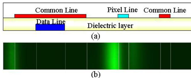
**FIGURE 1** — Light leakage due to crosstalk in the conventional IPS LC cell in the dark state: (a) the electrode structure, (b) calculated optical transmittance in the dark state.
