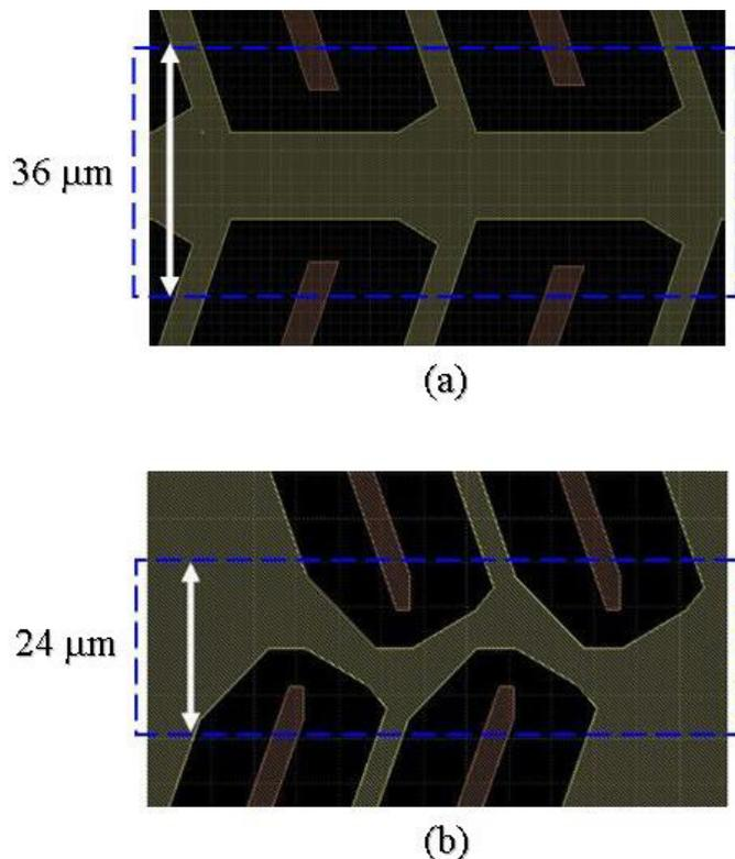
**FIGURE 6** — The structure of the electrode of the edge: (a) the conventional pattern, (b) the proposed zig-zag electrode pattern. The rectangular area with the blue line represents the required area for covering disclination. Dashed rectangle represents the required BM area.
