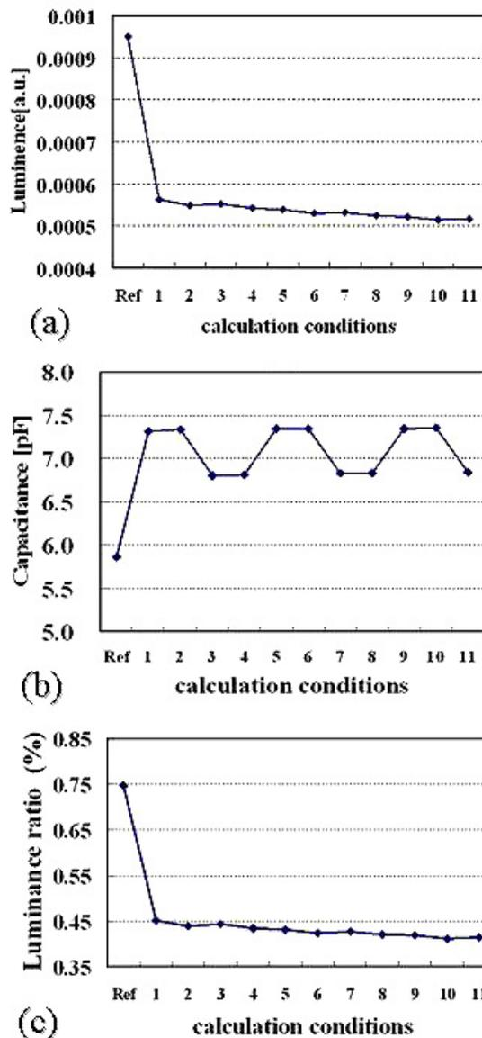
**FIGURE 3** — Calculated electro-optical properties related to the cross-talk: (a) light luminance in the dark state, (b) capacitance between the data line and the pixel line, (c) luminance ratio of the white and the black state.
