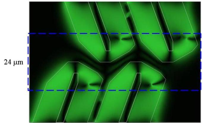
**FIGURE 7** — Calculated optical intensity on the proposed electrode pattern. Dashed rectangle represents the required BM area.
