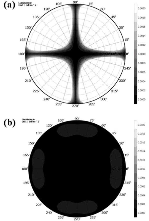
Fig. 4. Calculated iso-luminance in the dark state (a) for the conventional VA LC cell and (b) for the proposed VA LC cell.
