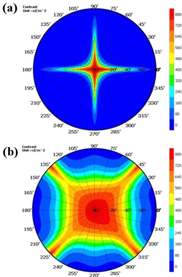
Fig. 5. Calculated iso-contrast contour (a) for the conventional VA LC cell and (b) for the proposed VA LC cell.
