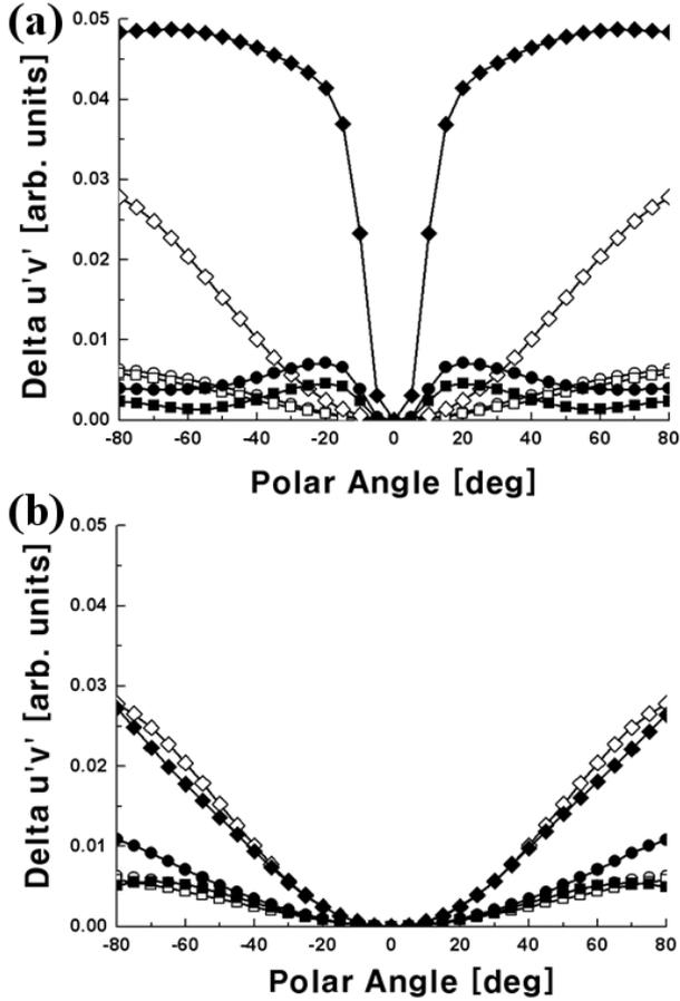
Fig. 3. Color shift for *R, G, B* wavelength light in the horizontal and the diagonal directions (a) for a conventional structure and (b) for the proposed structure. Symbols  $\circ, \square,$  and  $\diamond$  represent the *R, G, B* wavelength light in the horizontal direction, and symbols  $\bullet, \blacksquare,$  and  $\blacksquare$  represent the *R, G, B* wavelength light in the diagonal direction.
