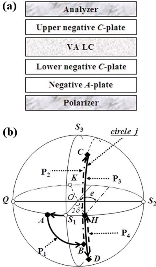
Fig. 2. Optical configuration and polarization states of the proposed VA LC cell: (a) optical configuration and (b) polarization path on the Poincaré sphere in the oblique incidence
