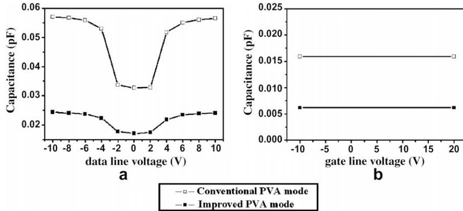
Fig. 8. Capacitance of the conventional and improved PVA modes: (a) capacitance of the common-data line (b) capacitance of the common-gate lines.
