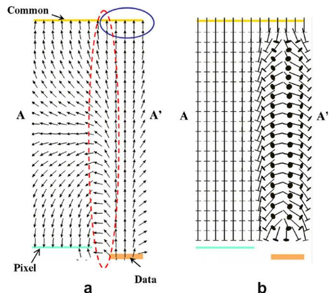
Fig. 3. (a) Electric field and (b) liquid crystal director distribution of the conventional PVA mode in the dark state.
