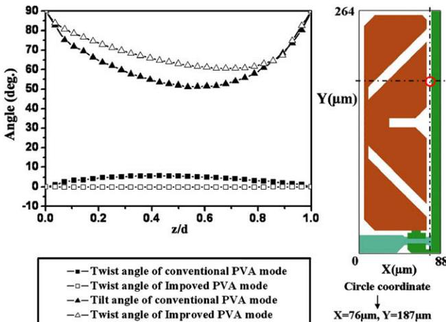
Fig. 5. Liquid crystal orientation in the tilt and twist angle of the conventional and improved PVA modes.
