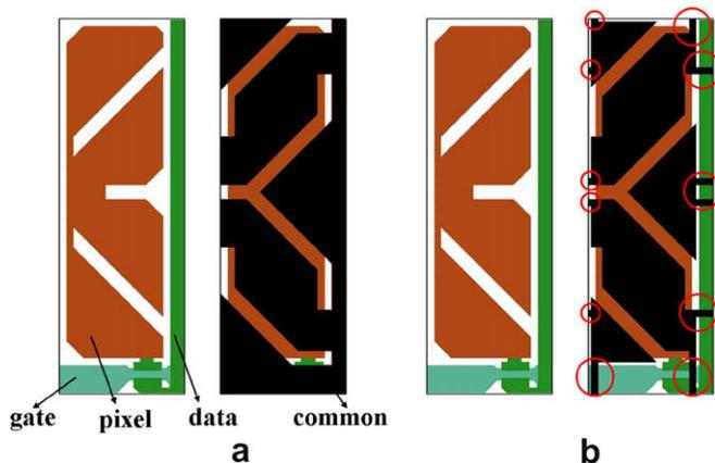
Fig. 1. Electrode structure of the PVA modes: (a) conventional and (b) improved PVA mode.
