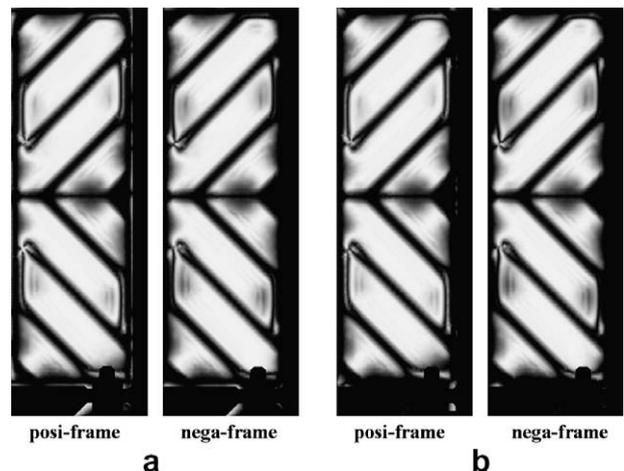
Fig. 7. Transmittance distribution at the operation voltage: (a) conventional and (b) improved PVA mode.
