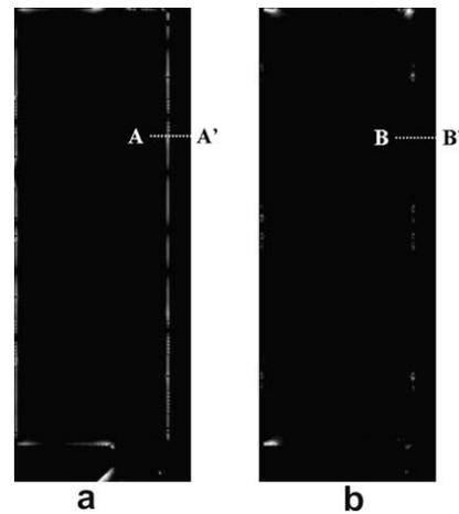
Fig. 2. Light leakage in the dark state: (a) conventional and (b) improved PVA mode.
