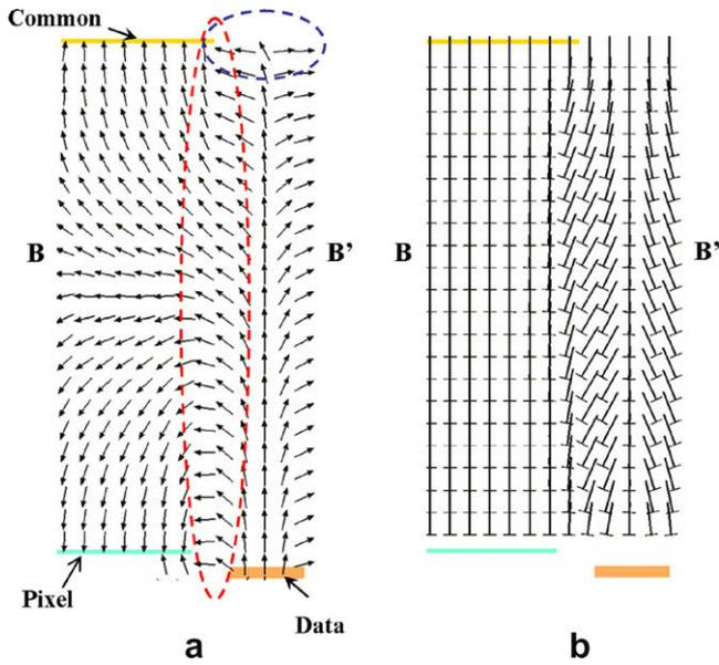
Fig. 4. (a) Electric field and (b) liquid crystal director distribution of the improved PVA mode in the dark state.
