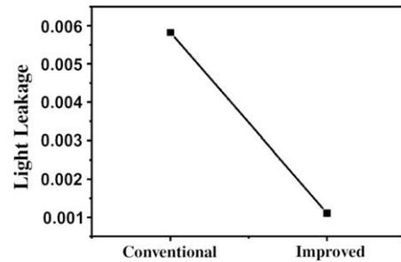
Fig. 6. Light leakage of the conventional and improved PVA modes at the normal direction in a dark state.
