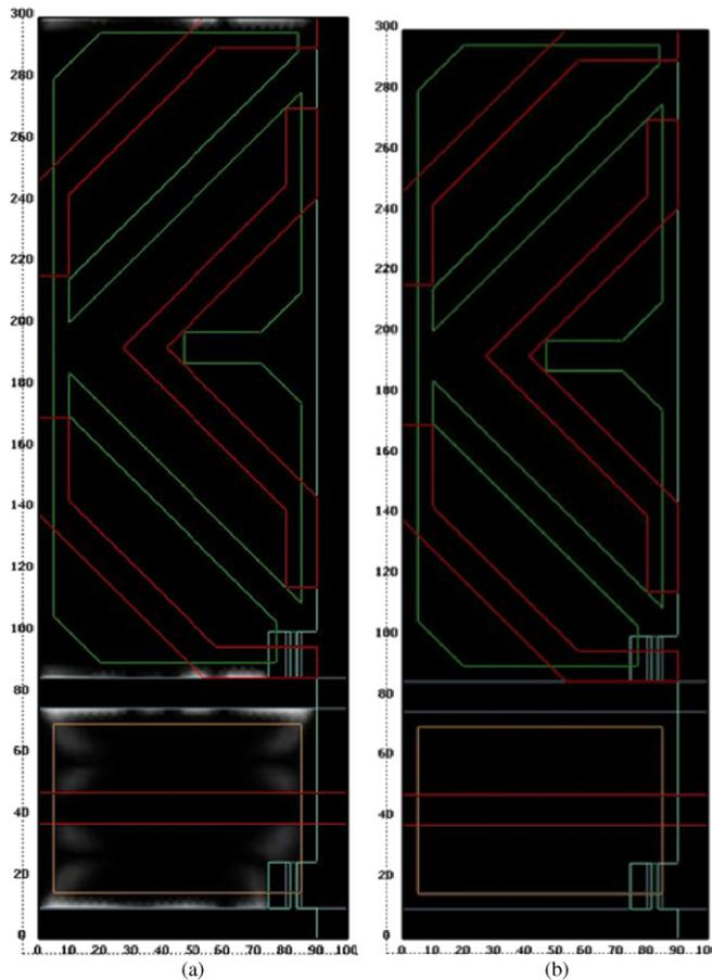
**Figure 4.** Light leakage of the controllable viewing angle PVA-LCD in the dark state: (a) narrow and (b) wide viewing angle modes.
