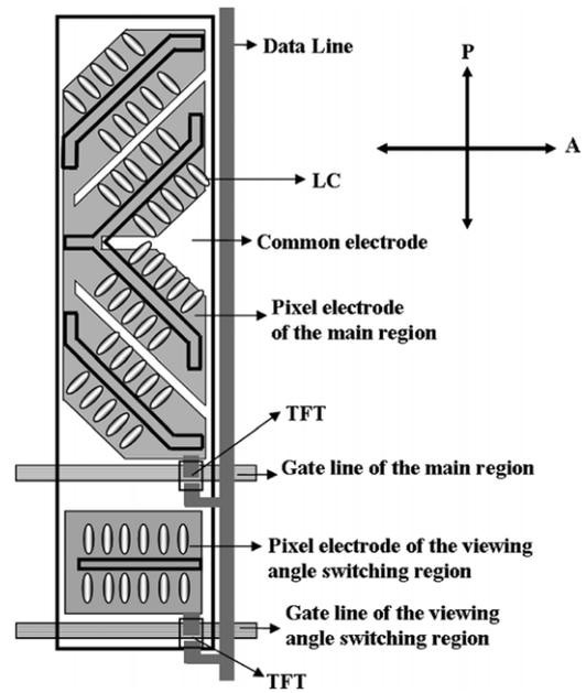
**Figure 2.** Electrode structure of the controllable viewing angle PVA-LCD with LC director direction in the on state.
