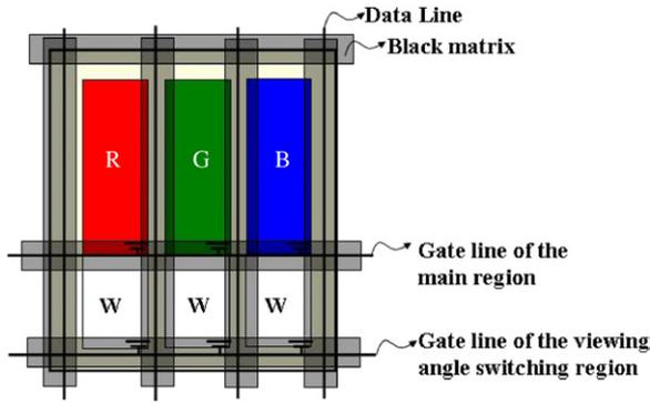
**Figure 3.** Arrangement of colour filter corresponding to figure 2. (This figure is in colour only in the electronic version)
