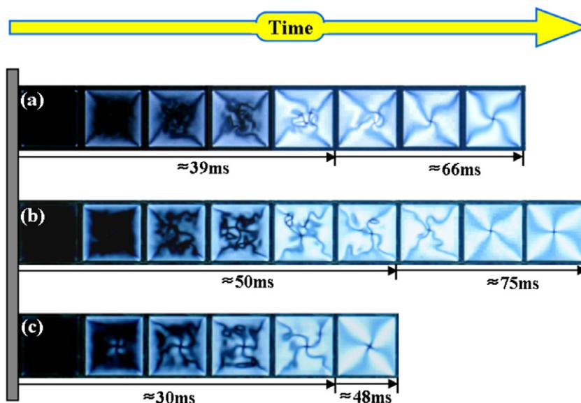
Fig. 7. Comparison of time-resolved textures when an operation voltage is applied to (a) C-1, (b) C-2, and (c) C-2 cell with removed part of upper electrode.
