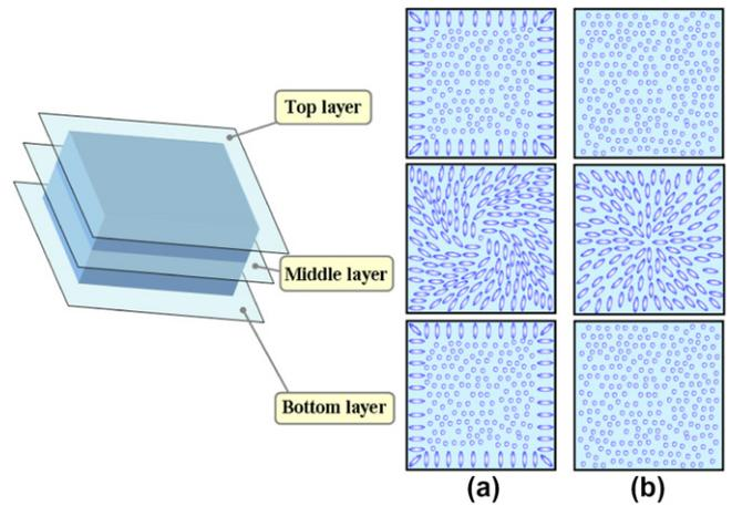
Fig. 5. Schematic two-dimensional orientation of LC in on state at three different vertical distances for (a) C-1 and (b) C-2 cells.
