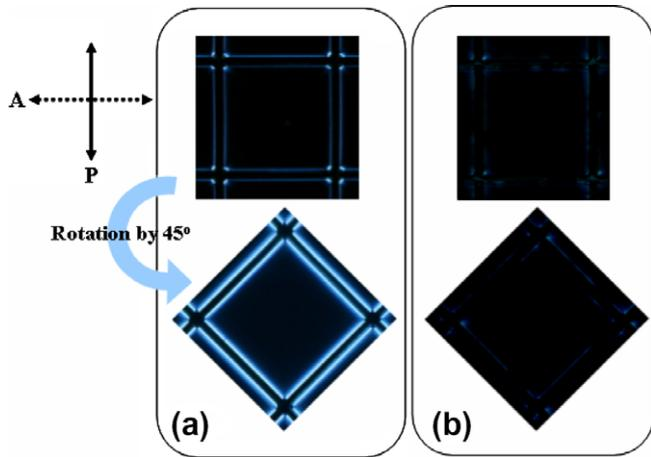
Fig. 4. The light leakage of a dark state in (a) C-1 and (b) C-2 near the polymer wall according to transmittance axis of crossed polarizer.
