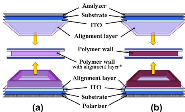
Fig. 1. Structures of (a) C-1 cell and (b) C-2 cell.
