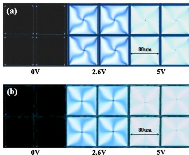
Fig. 3. Optical microphotographs of the LC textures at 0 V, 2.6 V, and 5 V in (a) C-1 and (b) C-2 cells.
