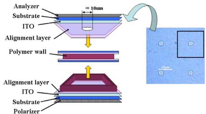
Fig. 6. Structures of C-2 cell with removed part of upper electrode.
