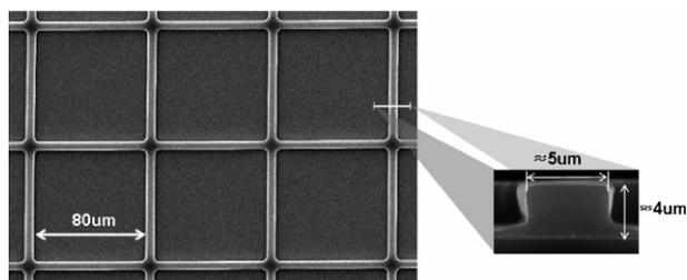
Fig. 2. Top-view and cross section of polymer wall on the bottom substrate.
