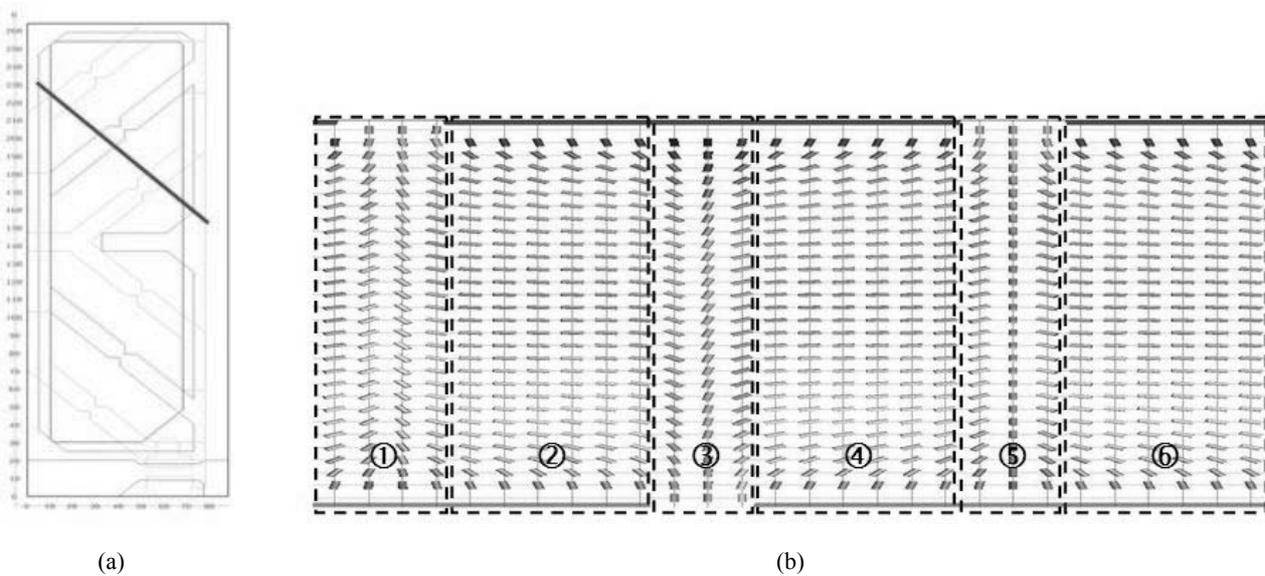
**Fig. 3.** (a) One pixel of the PVA LC cell, and (b) schematic cross-sectional view of the LC cell with the LC configuration in the bright state.
