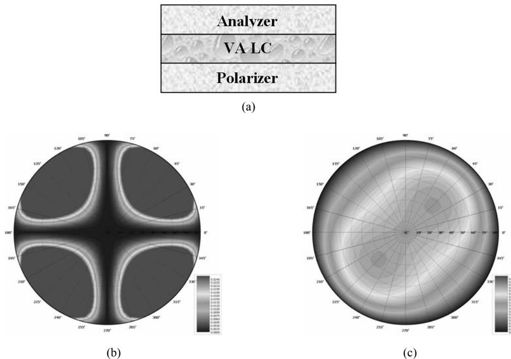
**Fig. 1.** Normal VA LCD with a uniform half-wave LC layer: (a) optical configuration, (b) iso-dark contour, and (c) iso-bright contour.
