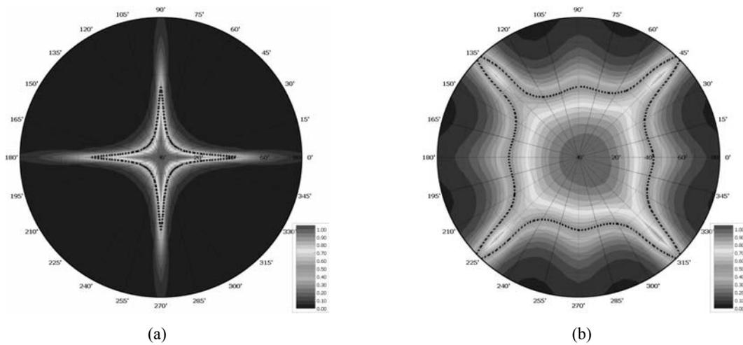
**Fig. 5.** Normalized iso-contrast contour with a non-uniform LC layer: (a) the normal PVA LC cell, and (b) the advanced PVA LC cell.
