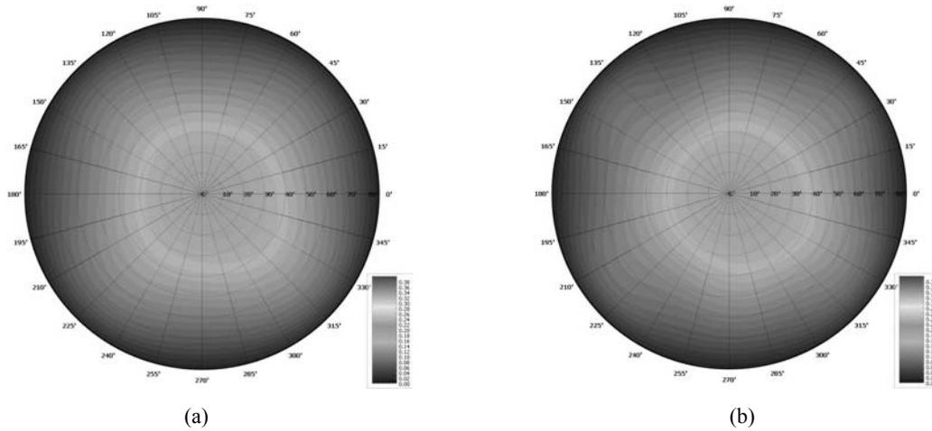
**Fig. 4.** Iso-bright contour of the PVA LC cell with a non-uniform LC layer: (a) the normal PVA LC cell, and (b) the advanced PVA LC cell.
