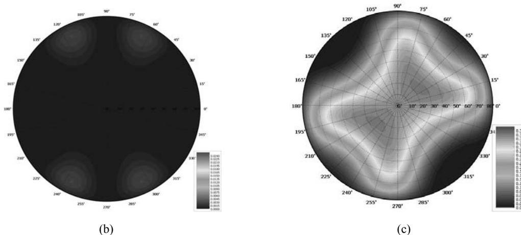
**Fig. 2.** Advanced VA LCD with a uniform half-wave LC layer: (a) optical configuration, (b) iso-dark contour, and (c) iso-bright contour.
