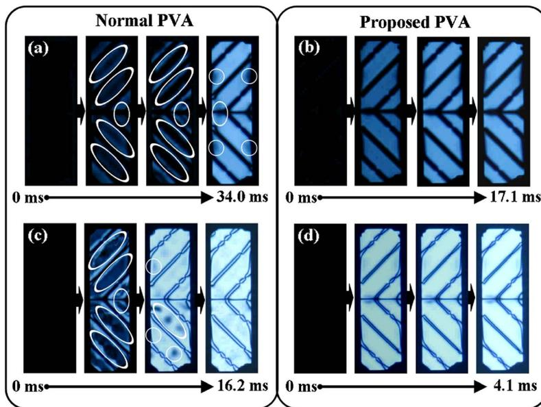
FIG. 4. (Color online) Comparison between normal PVA and proposed PVA for time-resolved LC textures and rising time: (a) and (b) are for  $T_{50}$  and (c) and (d) are for  $T_{90}$ , respectively.
