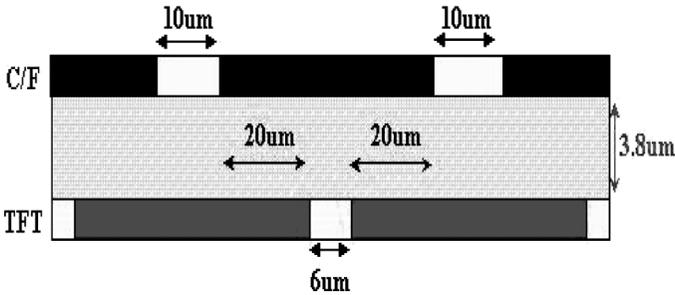
**FIGURE 1** The cell geometry used for the calculation.
