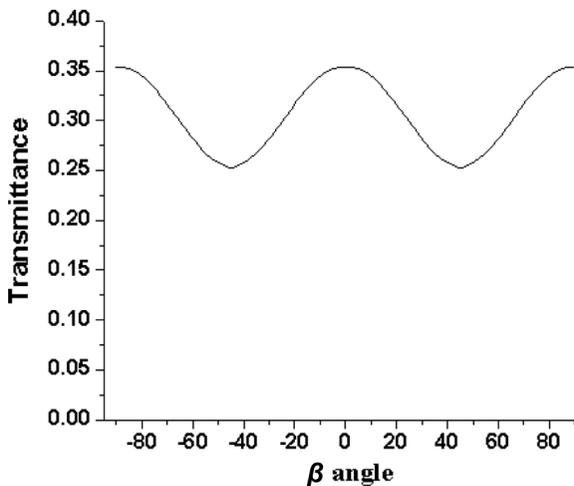
**FIGURE 5** Transmittance variation according to angle  $\beta$  in the VA-TN.
