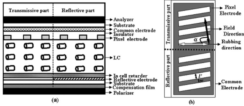
**Figure 1.** Electrode structure of the transfective display using FFS mode: (a) cross-section and (b) top view.
