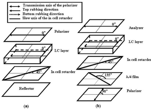
**Figure 2.** Optical configurations of the optical layers in the device: (a) reflective and (b) transmissive part.
