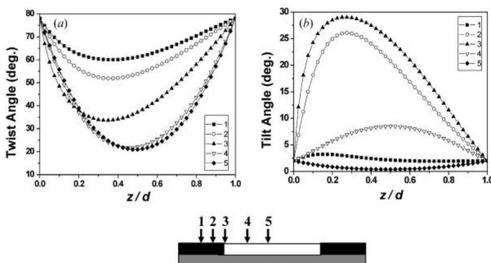
Figure 4. LC orientation (a) twist and (b) tilt angle in the white state along the vertical direction at several electrode positions.
