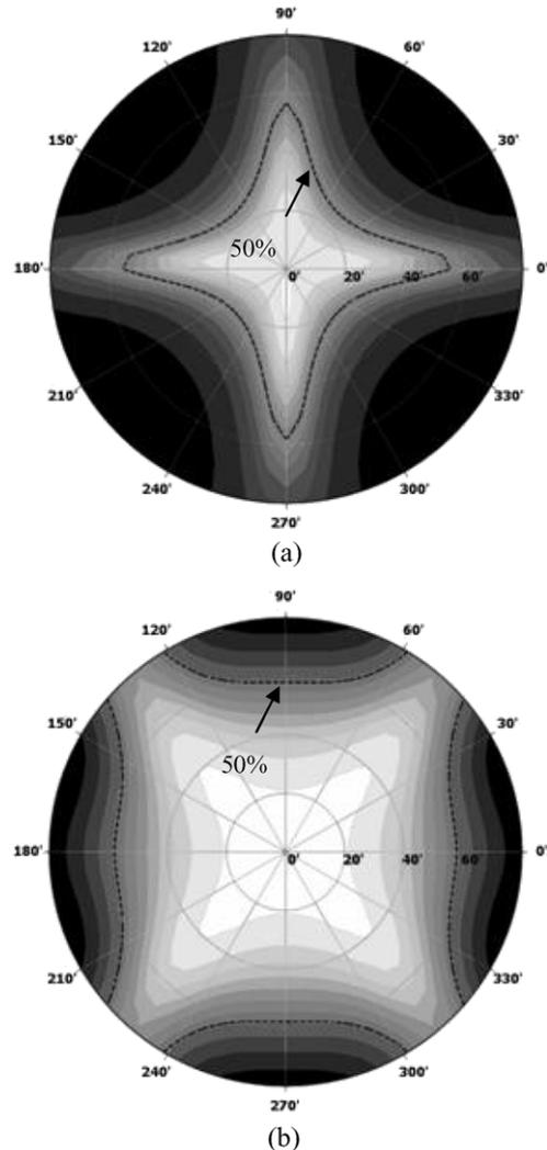
**Figure 6.** Normalized iso-contrast contour of the horizontal-switching cell. The dashed line represents the position of the half contrast ratio compared with the normal direction. (a) Conventional LC cell and (b) proposed LC cell.
