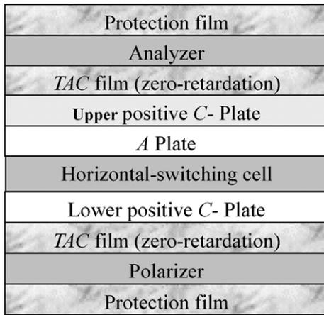
**Figure 2.** Optical configuration of the proposed horizontal-switching LC cell.
