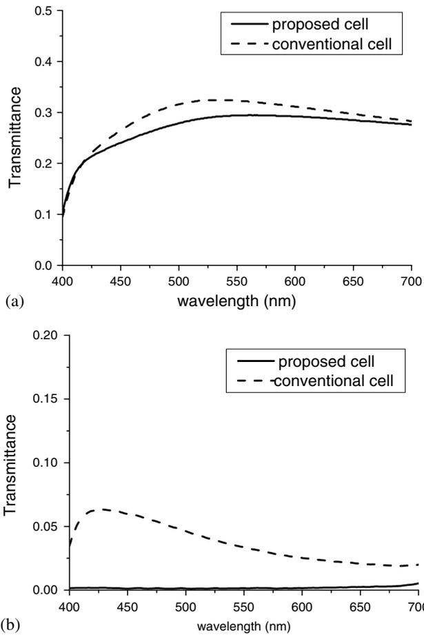
**Figure 5.** Comparison of optical transmittance of the proposed cell with that of the conventional cell; (a) in the bright state (b) in the dark state.
