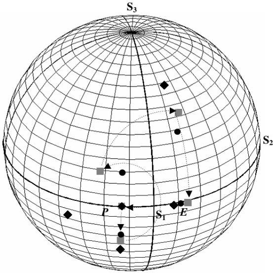
**Figure 4.** Calculated polarization states of the light passing through each retarder in the proposed LC cell on a Poincaré sphere ●, ■ and ◆ represent the polarization positions of red, green and blue wavelengths, respectively.
