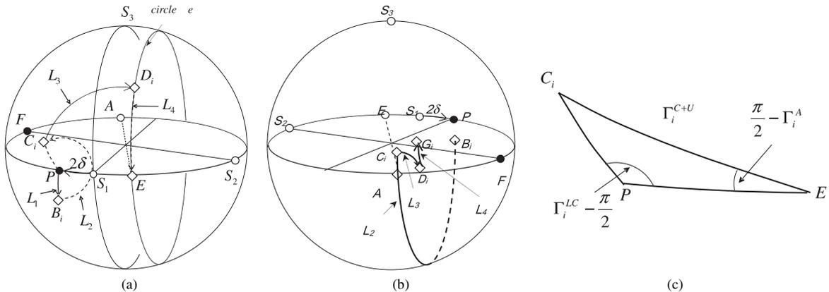
**Figure 3.** Polarization states of the oblique incident light in the proposed cell on the Poincaré sphere; (a) in the dark state, (b) in the bright state and (c) Trigonometric representation to remove the phase dispersion of the LC cell.  $L_1, L_2, L_3, L_4$  represent the transfer path of the polarization by the lower C-plate, the LC cell, A-plate and the upper C-plate, respectively. Subscript  $i$  represent the wavelengths R, G and B.
