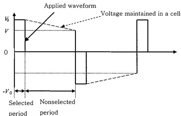
FIG. 6. Schematic drawing of the initial voltage ( $V_0$ ) applied during selected periods and the final voltage ( $V$ ) obtained by the relaxation of the liquid crystals during nonselected periods.
