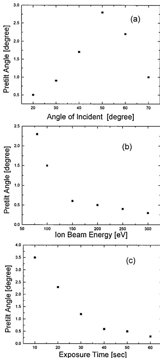
FIG. 3. The pretilt angle as a function of (a) the incident ion-beam angle, (b) the ion-beam energy, (c) the exposure time of the ion beam. SE-7492 was used as the polyimide.
