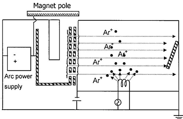
FIG. 1. Schematic drawing of an ion-beam system.
