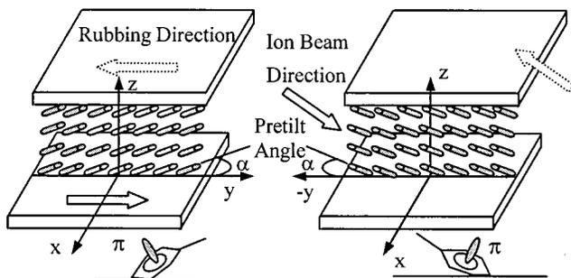
FIG. 2. Pretilt angles of a liquid crystal cell measured by the crystal rotation method in antiparallel cells fabricated by rubbing (left) and ion-beam-treatment (right). Pictures show that the tilted direction of liquid crystal cells is opposite to each other. The pretilt angle is determined by the direction of the  $\pi$  bond in polyimide.
