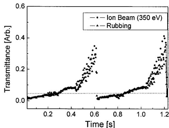
FIG. 7. Charge retention time measurement of TN cells fabricated by the rubbing method and the ion-beam method. The ion-beam energy: 350 eV, the incidence angle:  $45^\circ$ , and the exposure time: 25 s. The dotted line corresponds to the voltage holding of 90%.
