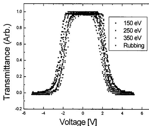
FIG. 4. Comparison of the voltage-transmittance curves of TN cells fabricated by the rubbing method and the ion-beam method. Then, the ion-beam energy: 150, 250, and 350 eV, the incidence angle:  $45^\circ$ , and the exposure time: 25 s.
