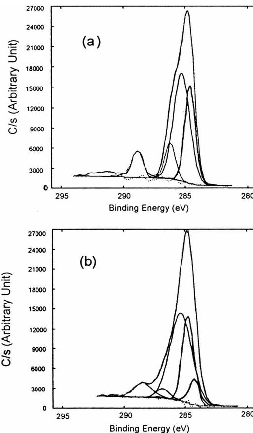
FIG. 5. Curve fitting of XPS data for SE-7492 as polyimide: (a) before the ion-beam exposure, (b) after the ion-beam exposure.
