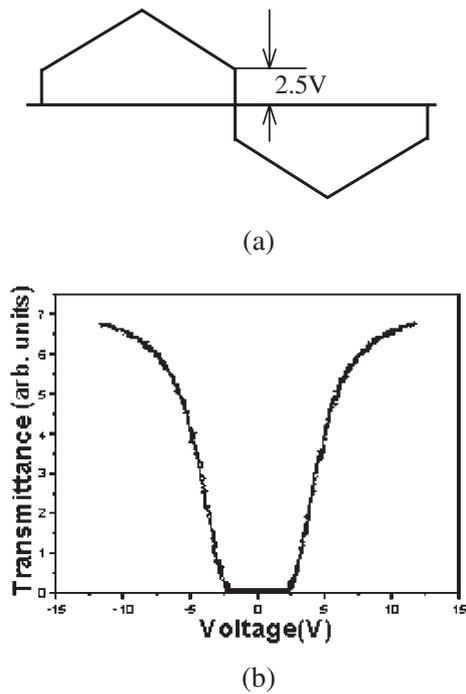
Fig. 2. (a) Triangular-wave form at a frequency of 5 Hz with a bias voltage of 2.5 V, (b) voltage dependence of transmittance in a  $\pi$  cell.
