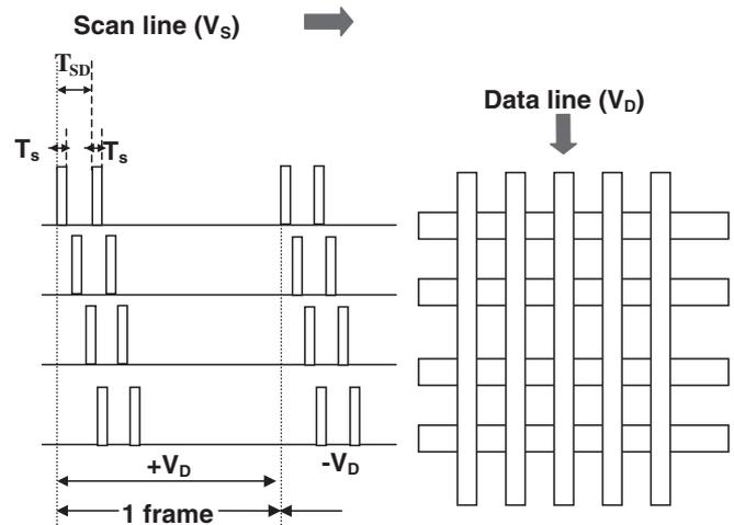
Fig. 1. Scan pulse of the proposed driving method.  $T_s$  is determined by the resolution and  $T_{SD}$  is the time between the first and second scan pulses.
