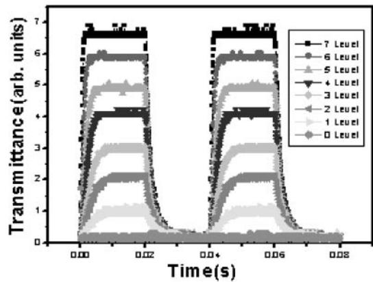
Fig. 5. Response characteristics of the  $\pi$  cell for the transitions from gray level zero to higher gray levels driven by the conventional driving method.
