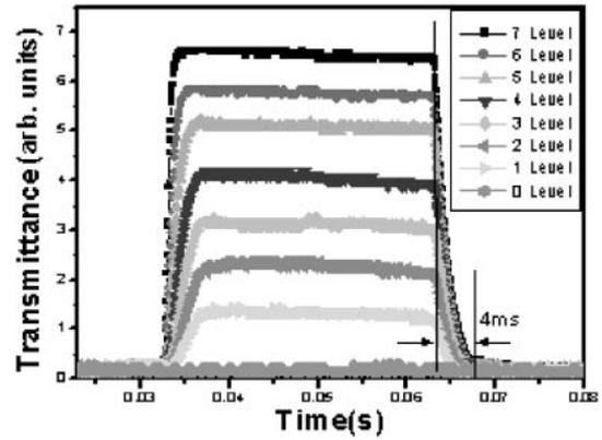
Fig. 8. Response characteristics of the 8 gray levels obtained by the proposed new driving method with  $T_{SD}$  of 4 ms.
