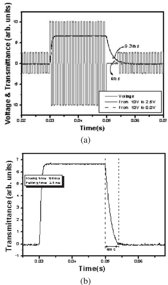
Fig. 3. Response characteristics of the transmittance with the applied voltage for the  $\pi$  cell: (a) Response characteristics for the applied voltage changes from 10 V to 2.5 V and 0 V, (b) enlarged response characteristics for measuring the response time, where the rising and falling times are 0.6 ms and 2.4 ms, respectively.
