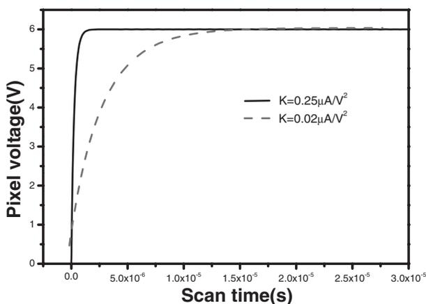
Fig. 7. Pixel voltage dependence on scan time calculated from the equivalent circuit.  $K = 0.25 \mu\text{A}/\text{V}^2$  and  $K = 0.02 \mu\text{A}/\text{V}^2$  are the values for the poly-Si TFT and a-Si TFT, respectively.
