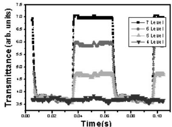
Fig. 9. Response characteristics for the transitions from gray level 4 to higher gray levels. All switching are also achieved within  $T_{SD}$  of 4 ms.
