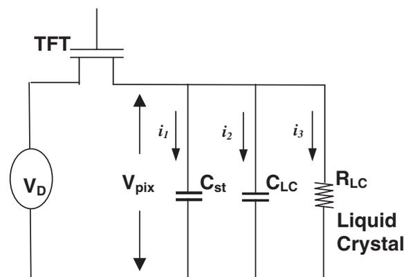
Fig. 6. Equivalent circuit of nematic liquid crystal cell.
