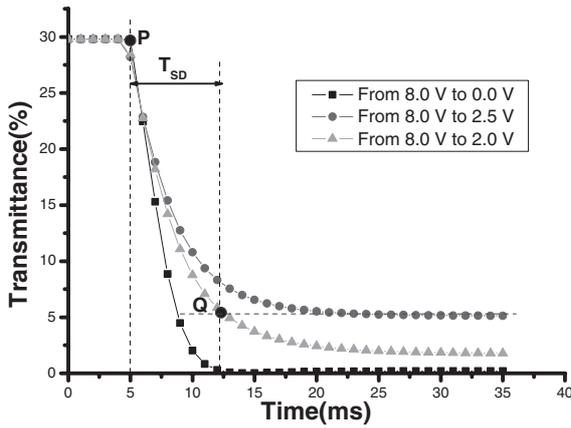
Fig. 4. Response characteristics of a  $\pi$  cell with a gap of  $5\ \mu\text{m}$  simulated for the applicability of the double scan method.
