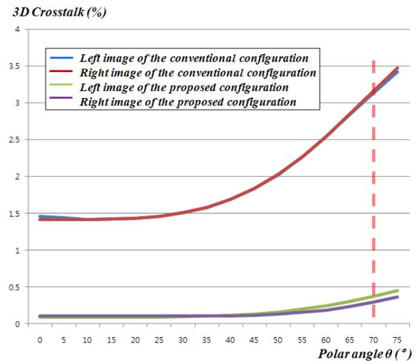
Fig. 4. Comparison of the calculated 3D crosstalk of the conventional and proposed configuration for the left and right image
