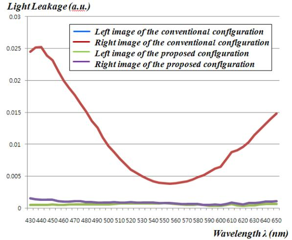
Fig. 3. Comparison of the light leakage for the conventional and proposed configuration in vertical direction ( $\theta=70^\circ$  and  $\varphi=90^\circ$ )
