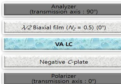
**Fig. 1 Configuration of conventional single domain VA LC cell**
