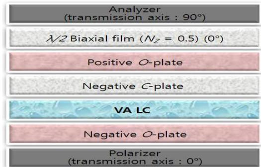
**Fig. 3 Configuration of proposed single domain VA LC cell**
