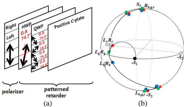
**Fig.2. (a) Proposed configuration of patterned retarder (b) polarization states of the left ( $L_{i=r, g, b}$ ) and right ( $R_{i=r, g, b}$ ) image in horizontal viewing angle**
