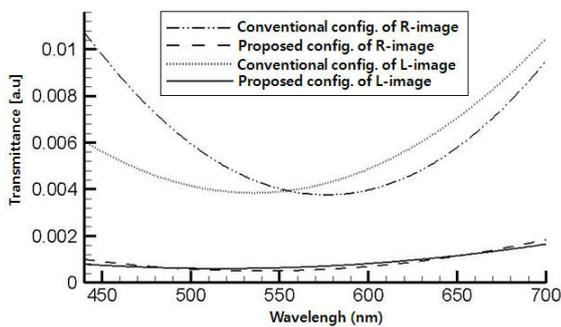
**Fig.3. Comparison of the light leakage between the conventional and the proposed configuration for left and right image in horizontal direction**
