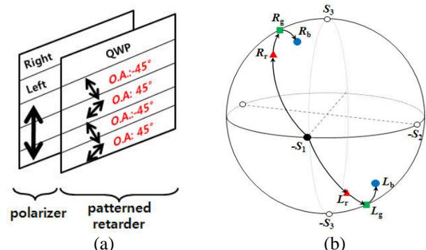
**Fig.1. (a) Conventional configuration of patterned retarder (b) Polarization states of the left ( $L_{i=r, g, b}$ ) and right ( $R_{i=r, g, b}$ ) image in horizontal direction**
