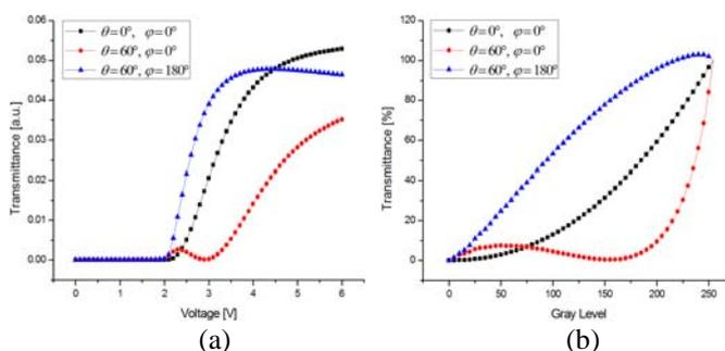
**Fig. 2. The V-T curve and Gamma curve properties of the conventional VA LC cell: (a) V-T curve (b) gamma curve.**
