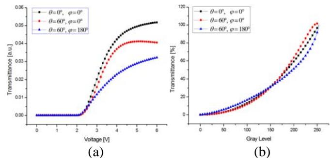
**Fig. 5. The V-T curve and Gamma curve properties of the proposed VA LC cell: (a) V-T curve (b) gamma curve.**
