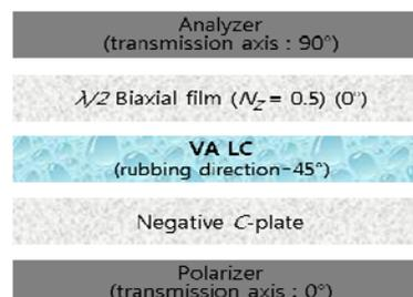
**Fig. 1. Optical configuration of the conventional VA LC cell.**
