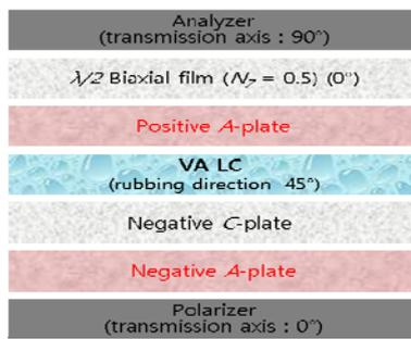
**Fig. 3. Proposed optical configuration of the VA LC cell .**
