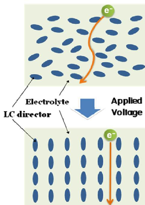
Fig. 1. Before and after of electron transportation according to LC alignment
