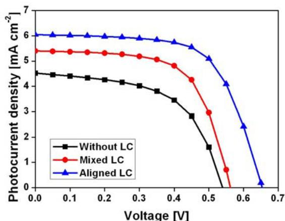
Fig. 2. J-V curve under A.M 1.5G 1 sun illumination (100mW/cm<sup>2</sup>)
