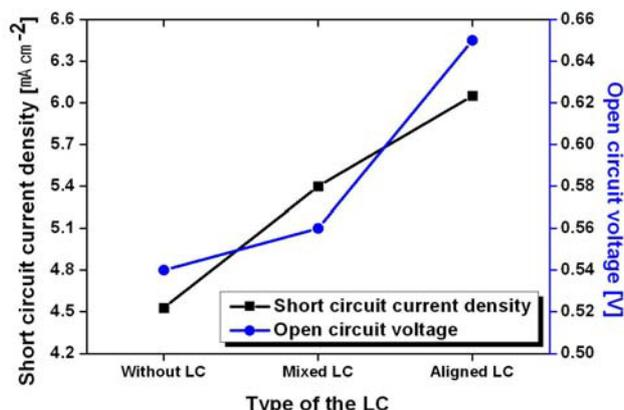
(a) Open circuit voltage ( $V_{OC}$ ) and Short circuit current density ( $J_{SC}$ ) according to type of the LC
