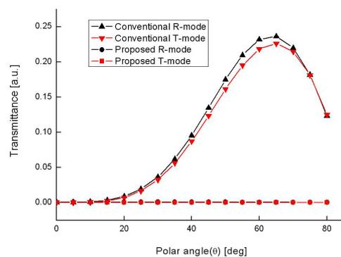
**Fig. 3. Comparison of the transmittance between the conventional and the proposed CPs as a function of the polar angle at  $\phi = 45^\circ$  in the dark state**
