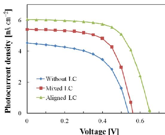
**Fig. 2. J-V curve under A.M 1.5G 1 sun illumination (100mW/cm<sup>2</sup>)**
