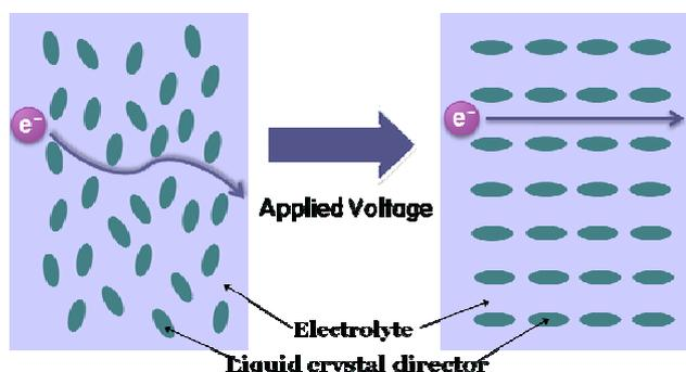
**Fig. 1. Comparison of electron transportation according to LC alignment**
