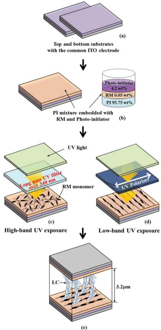
**Fig. 2 Schematic diagram of the fabrication process of the proposed two-band UV exposure system for enhancing the surface anchoring energy of the photo-sensitive PI layer**
