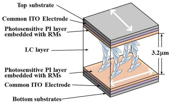
**Fig. 1 The modeled optical configuration of the TN LC cell for experiments**
