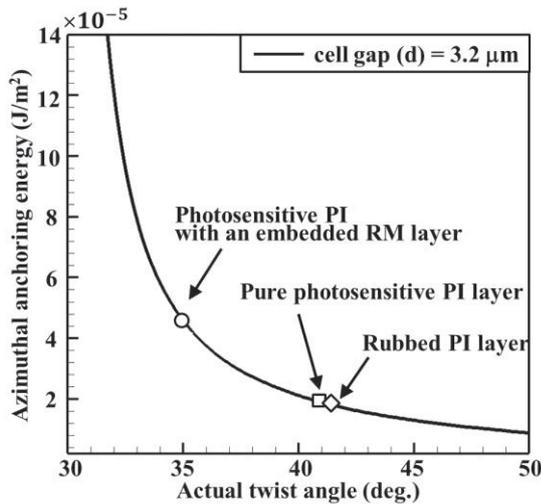
**Fig. 3 Comparison of the measured surface anchoring energy for three PI samples: the rubbed PI layer, the pure photo-sensitive PI layer and the proposed photo-sensitive Pi with an embedded RM layer**
