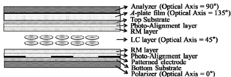
Figure 1. Optical configuration of the proposed RF IPS LC cell with Photo alignment layer.
