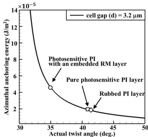
**Figure 1.** Comparison of the measured surface anchoring energy for three PI samples.
