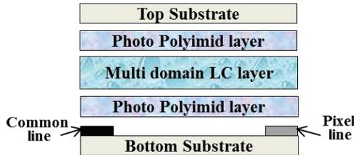
**Fig. 2. The cross-sectional view of the cell structure for fabricating the proposed IPS LC cell**
