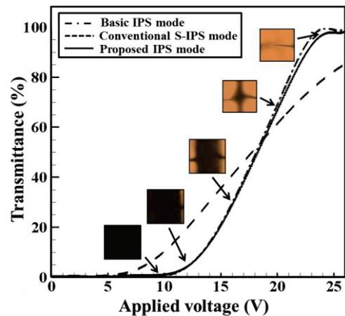
**Fig. 5.** The comparison of the calculated voltage-transmittance (V-T) curve in a basic IPS mode, a conventional S-IPS mode and a proposed IPS mode including the measured optical intensity of the LC cell.
