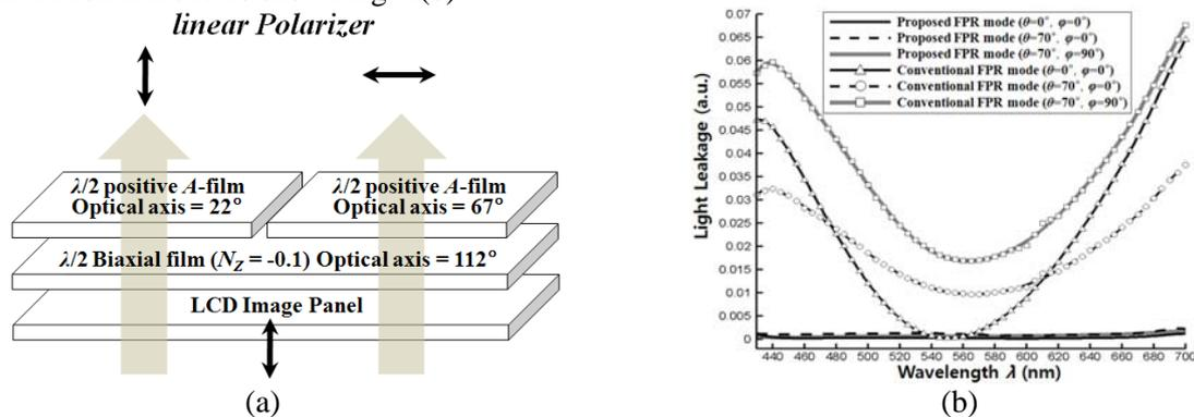
Fig. 1. (a) The optical configuration of the proposed FPR cell. (b) The comparison of the calculated light leakage of conventional and proposed configuration in each viewing angle.
