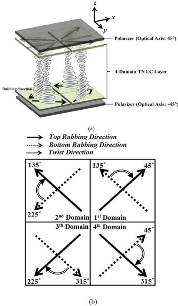
Fig. 1. (Color online) A conventional 4-D TN LC cell: (a) the optical configuration and (b) the twisted LC director configuration in each domain.
