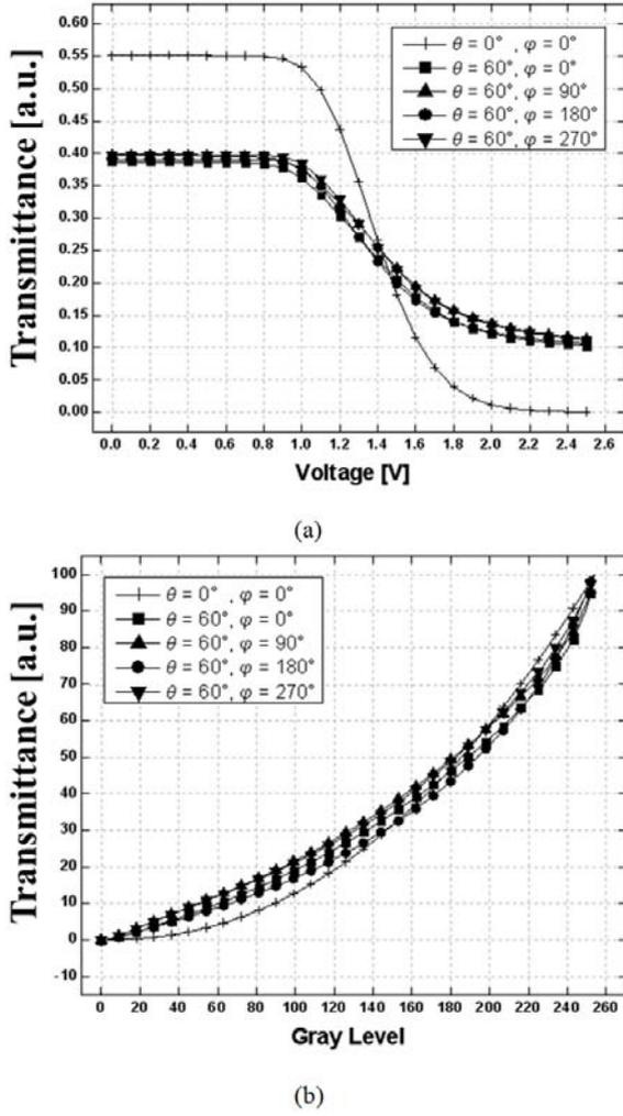
Fig. 5. The calculated (a) V-T curve and (b)  $\gamma$ -curve of the proposed 4-D TN LC cell for all viewing angles.
