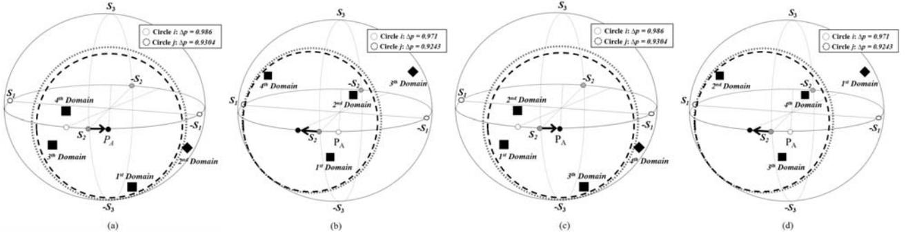
Fig. 3. The polarization positions of each domain in a conventional 4-D TN LC cell under an applied voltage of 2.2V in the oblique direction with azimuth angles of (a) 0°, (b) 90°, (c) 180° and (d) 270°.
