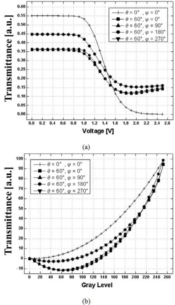
Fig. 2. The calculated (a) V-T curve and (b)  $\gamma$ -curve of the conventional 4-D TN LC cell on-axis ( $\theta = 0^\circ$ ,  $\phi = 0^\circ$ ) and off-axis ( $\theta = 60^\circ$ ,  $\phi = 0^\circ, 90^\circ, 180^\circ$  and  $270^\circ$ ).
