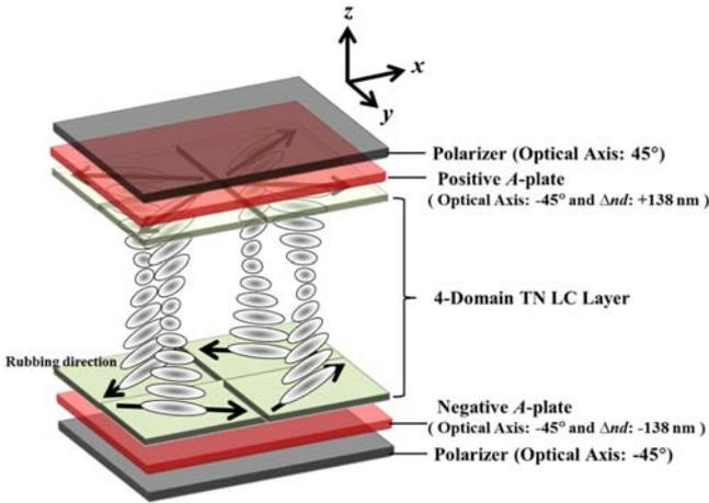
Fig. 4. (Color online) The proposed optical configuration of the 4-D TN LC cell.
