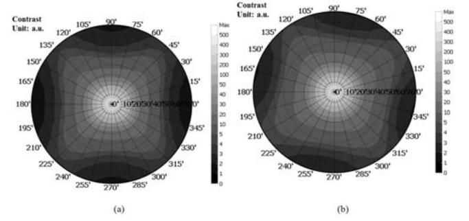
Fig. 6. Comparison between the iso-contrasts of (a) a conventional 4-D TN LC cell and (b) the proposed 4-D TN LC cell.
