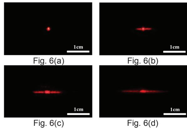
**Fig. 6.** The measured refracted light width at the observing distance (=30 cm) of the proposed PPLC lens (a) at 0 V, (b) at 40 V (~ 0.8 cm), (c) 100 V (~ 1.3 cm), and (d) 130 V (~ 2 cm).
