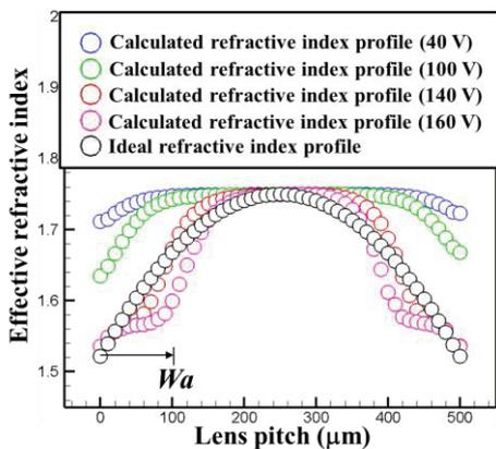
**Fig. 5.** Calculated effective refractive index profile of the LC lens layer in 3D mode.
