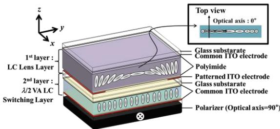
**Fig. 2. The proposed 2D/3D switchable PPLC lens structure**
