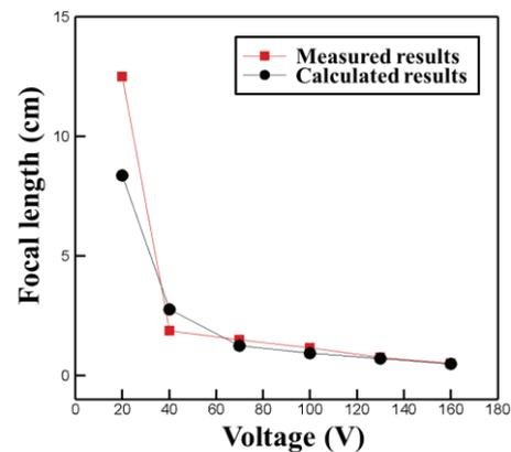
**Fig. 7.** The comparison of the focal length of the calculation and measurement in the proposed PPLC lens.
