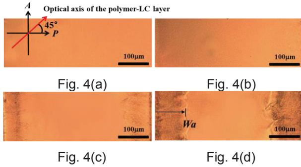
**Fig. 4.** The microscopic image of the fabricated LC lens layer at the applied voltage state of (a) 0 V, (b) 40 V, (c) 100 V, and (d) 160 V, respectively.
